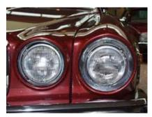
Two round lights on a side, with one in the fender (wing), and one in the hood (bonnet) such that it points down when open.
