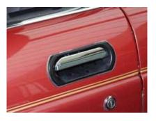
Ovoid, metal. Lock mechanism mounted in door separately.
