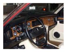
Aircraft-style, with four smaller gauges flanking two large ones.
