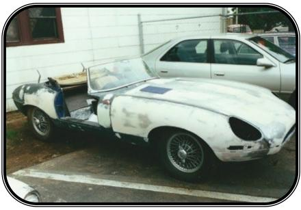
Looking it over it appeared to be all there, but in very rough condition (little did I know how rough!). The paint was crazed and chipped. The original color was BRG but the next layer red and finally blue. The interior was completely shot, seats, carpets and the dash were torn and cracked, the windshield broken and some switches missing. Driving it didn't get better. Brakes worked
